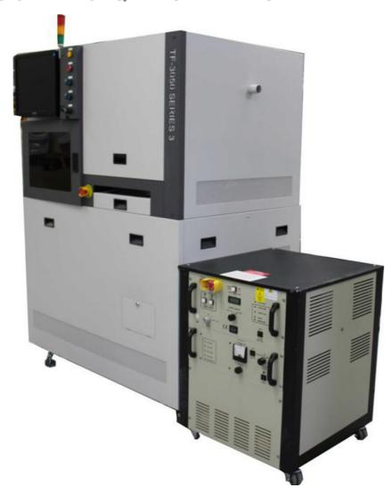
The **TF-3050 Series 3 LDP10TQ** provides high accuracy performance to overcome the new challenges of smaller geometries of chip resistor trimming. Proprietary designs achieve the high accuracy mechanical positioning and ultra-stable laser beam control demanded by industry. **TF-3050 S3** utilizes vision registration theta rotation within a Windows XP operating system. These advance features are integrated with established substrate handling and automation systems.
